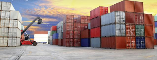
Cargo Transport Units (CTUs) are designed with the intention of being versatile due to the requirement to adapt to a variety of modes of transport. They do so by being rolled or lifted from one form of transport to another. A swap body can be carried on a road vehicle or railway wagon. A deep sea container can be carried on a road vehicle, railway wagon, inland barge or seagoing vessel for example.
